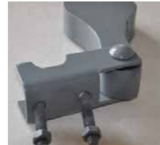
Discharge Rapping Hammer
