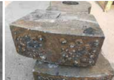
Hammer With Insert Alloy
